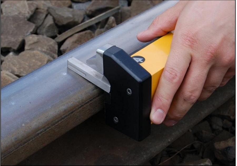
Fig. Nr. 4.3 Measuring the guiding surface of the rail
