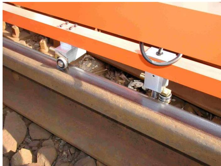
Figure 2 Longitudinal measuring frame with the radius of curvature and sinking measuring units.
