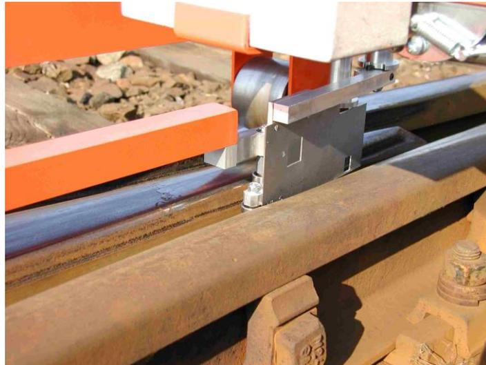
Figure 1 Pass of the measuring device during measuring minimum flangeway and maximum check-rail gauge.
