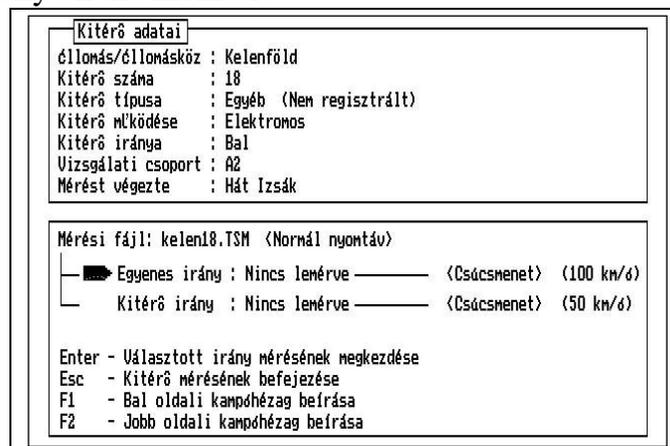
Figure 6 The measuring programme data field interface
