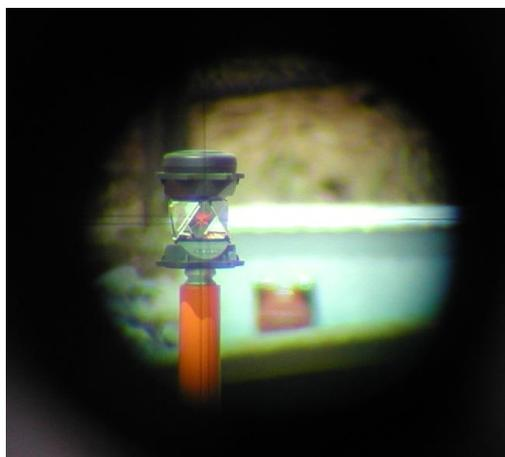
Figure 4 The prism through the measuring station
